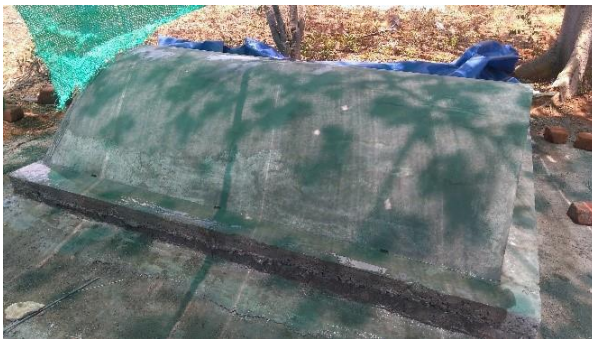
3. Base Mould for fabricating circular slabs side view
